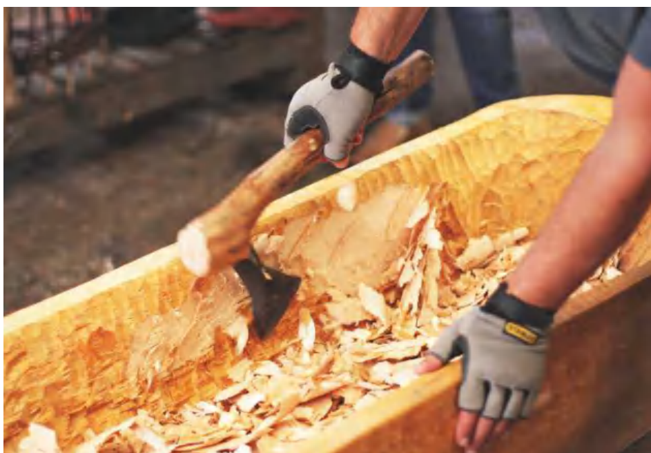
▲ Shaping the inside with an axe
